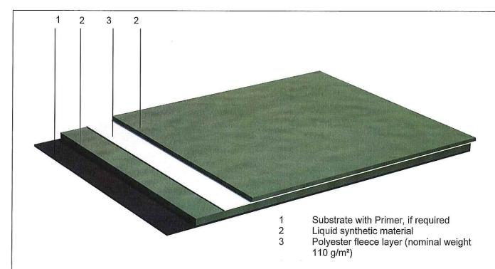
Applicable to the roof waterproofing "Renolit Poliquid Infinite", "Renolit Poliquid Detail" and "Renolit Poliquid Infinite MX":
